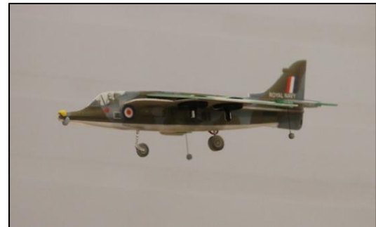
John Whatmore's Harrier is from 2mm Depron with electronics from an Eachien E010 micro quad. AUW not including battery is 20.4 grams [photo by Andy B]
