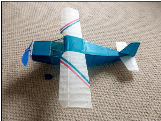
Own-design Nesmith-Cougar-based Bostonian by Dave King, weighs 19.5 grams [Dave King photo]
